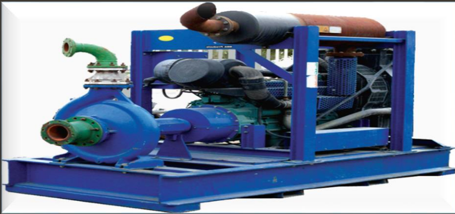
CENTRIFUGAL PUMP: CAPACITY : 800, 400 ,200, 60 , 20 M 3 / hr
